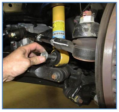
3. Disconnect tie rod – Remove the cotter pin, then remove the nut using a 22mm wrench or socket. Separate the tie rod from the knuckle.
