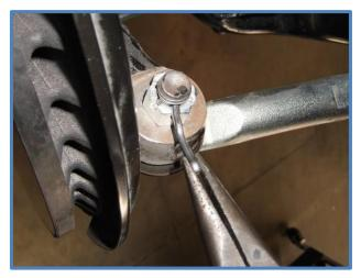
6. Remove lower mounting bolt using a 19mm wrench and socket.
