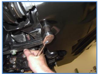
15. Now remove the sway bar mounting bolts at the frame using a 14mm socket. Do one side at a time.
