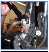
Use an allen wrench to hold the sway bar link stud for removing and tightening nut.
