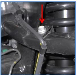
4. Remove Sway Bar, notice that the sway bar mounting brackets are side specific and must be oriented properly when reinstalling.
