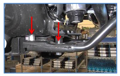
12. Install skid plate using the factory hardware.
