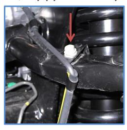
3. Keep a jack under the lower control arm on the side you are working on while disconnecting suspension components. Disconnect upper A-arms (A), tie rods (B), and lower shock mounting bolts (C).
