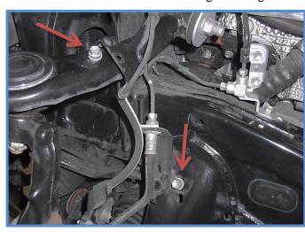
4. Remove the three nuts from the upper mount, lower the jack and remove shock. Remove shocks from both sides before attempting to install new shocks.
