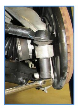
a 21mm socket, loosen the nut on the A-arm ball joint. Separate the ball joint from the upright using proper ball joint tools.
