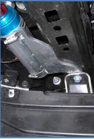
**NOTE:** 2wd — For 2wd models and/or vehicles without tow hooks you may need to remove bumper to install reservoir brackets if access to mounting points is not available. Use the supplied 10mm hardware to attach brackets to existing holes in frame if tow hooks and tow hook hardware are not installed on your vehicle.
