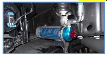
11. Using a 9/16" socket, torque the 3/8" upper shock mount bolts to 35ft/lbs. Torque the lower shock bolts to 75ft/lbs. using an 18mm & 19mm wrench/socket.
