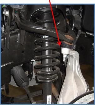
4. Remove the nuts from the lower shock mount using an 18mm socket. Save the nuts you will
