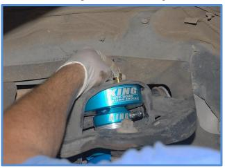
4. Install the factory bolt in the lower mount and tighten to factory specs. You can now tighten the three upper mounting bolts to 35 ft/lbs.
