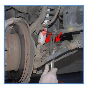
2. Remove the three nuts from the upper mount and remove shock from vehicle.
