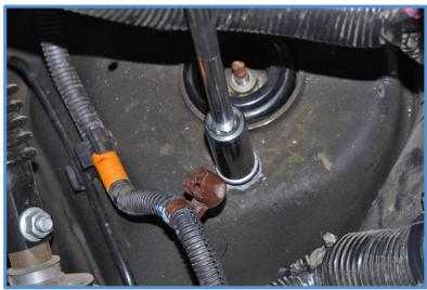
3. Using a 15mm socket, remove the lower shock mount bolts then remove the factory shock.
