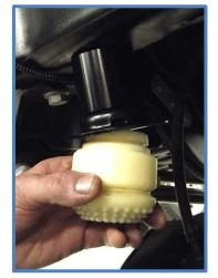
8. Remove the lower coil mount using an 18mm Socket.
