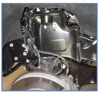
4. Remove the foam bump stop from the mount on frame. Pull the bump stop to the side and down with a firm tug to remove bump stop.
