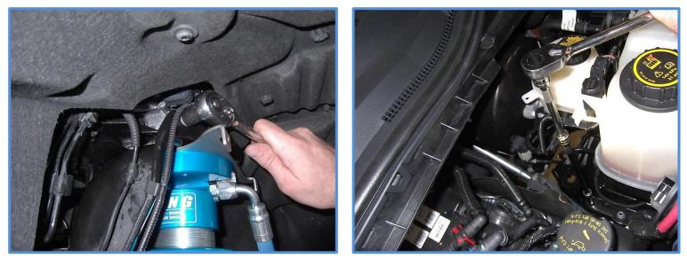
18. For 2.5 kits with standard reservoir, place the reservoir in the reservoir bracket and install the provided hose clamps. Center the reservoir in the cradle and twist the reservoir towards you to twist the hose in towards the wheel well and tighten the clamps.
