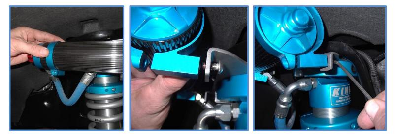
20. Center reservoir in the bracket and insert the provided 1" socket head cap screws in the clamps and tighten with a 3/16 allen wrench to secure reservoir. Hose should be pointing back as shown below.
