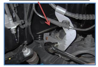
3. With the shocks removed and the ABS/brake lines disconnected, lower the axle and remove the coil springs.
