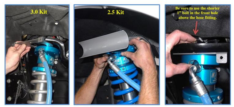
16. Install upper mounting bolts and tighten to 35 ft.lbs. using a 9/16 wrench/socket.
