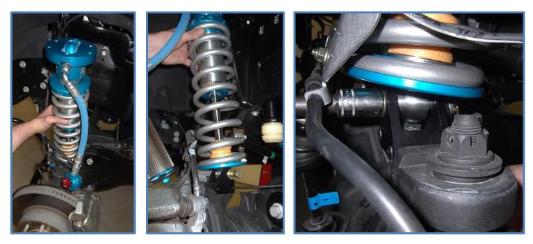
14. On the left side of some vehicles you will need to move the brake proportioning unit to install the upper mounting bolts. First remove the bolt on the front side of the coil mount using a 13mm wrench/socket. Then find the two nuts located inside the engine compartment and just loosen those nuts to the end of the stud but do not remove. This should give you room to pry the brake unit up enough to install bolts.
