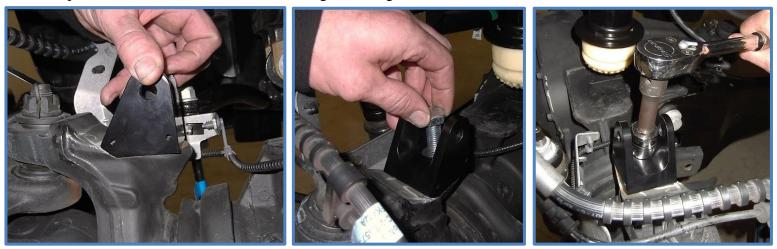
10. Using the reservoir bracket as a template carefully mark the holes in the upper coil spring mount. Mark holes, then center punch each hole and recheck the alignment of marked holes with reservoir bracket. (For customers who received a reservoir bracket with slotted holes you should also have a paper template. Make sure paper template matches the hole pattern on the King upper mounting plate. Cut out template and use paper template to mark holes.)
