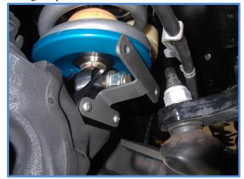
22. Attach the brake line to the previously installed brake line support by placing the tab in the inward hole and install the <sup>1</sup>/<sub>4</sub> x <sup>3</sup>/<sub>4</sub> bolt with washer in the outward hole making sure the head of bolt is on the same side as shock. Install washer and nut and tighten with 7/16 wrench and socket.
