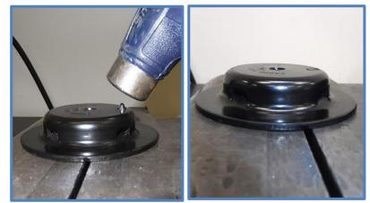
7. Reinstall the bump stop mount with the supplied spacer and longer bolt w/washer. Tighten the bolt using a 6mm Allen wrench. Push the bump stop back into the mount making sure it's pushed in all the way.
