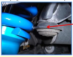
Rotate the bump stop pad or grind any material making contact with the shock at full droop.
