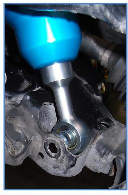
9. Line up the holes in the upper mounting plate on coilover with the upper mount on the vehicle and use the supplied 3/8 X 1" HHCS (CB4701) and 3/8 SAE HD Washers (CW1701) to attach the new coilover to the factory upper mount. Using a 9/16" socket, torque the 3/8" upper shock mount bolts to 35ft/lbs.
