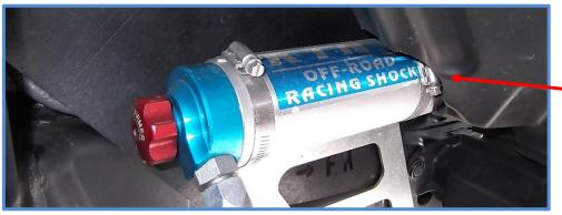
Some vehicles may require plastic trimming in the inner fender well to mount reservoir.
