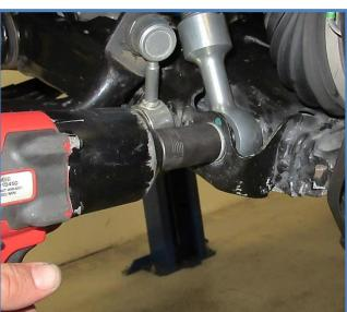
11. Check clearance at full droop, you may need to simply rotate the bump stop using a large wrench or channel locks. On some vehicles you may need to grind the bump stop bracket or HEX portion of the pad so the spring does not contact at full droop.
