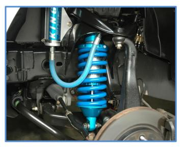
6. Once the shock is in and secure, slide the reservoir into the reservoir bracket and secure it with both hose clamps. (make sure the reservoir is centered in the bracket)
