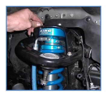
8. Install reservoir in the reservoir bracket using the provided hose clamps. Position the reservoir so it is centered in the cradle with the hose pointing straight back. Adjust accordingly.
