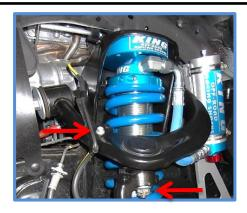
10. Install the sway bar to the threaded holes in the reservoir bracket using the 3/8"x 3/4" bolts and washers provided in the kit. The factory sway bar brackets are side specific and stamped "L" and "R" with an arrow that points toward the front of the vehicle. After the sway bar is mounted to the frame you can reconnect the sway bar links to the steering knuckle upright.
