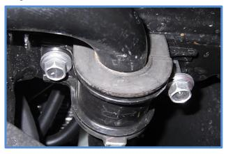
16. Slide the base of the reservoir bracket between the sway bar and the frame. Use the provided M10-1.25 X 40mm SHCS (CB1804) to mount the reservoir bracket to the existing holes in the frame. Tighten bolts to 30 ft-lbs using an 8mm (or 5/16) Allen wrench.
