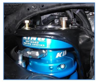
9. Place the rod end in the lower mount and install the factory bolt. Tighten lower bolt to factory specs. Now you can torque the upper mounting bolts to 35 ft/lbs.
