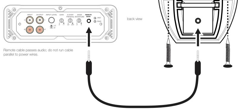
Connect the supplied 1/8th inch [3.5mm] patch cable to the CXARC remote and the Remote Bass jack on the amplifier.
