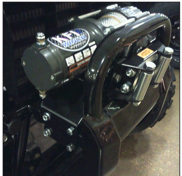
“Figure 8 Winch and Mount Installed”
