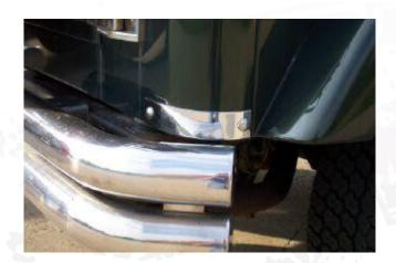
Place the rear corner guard in place and align the bottom edge of the guard with the body tub. Mark the two mounting holes with a magic marker. Center punch the mark, then drill with a small drill bit. Re-drill the holes using an 11/32" drill bit. Bolt the corner guards in place using the stainless steel bolts provided.
