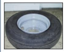
Break and lube both beads. Lay tire on floor with short side of wheel up.
