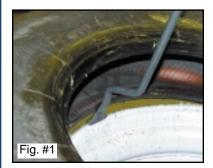
**Mounting:** Insert valve stem. Lubricate both bead seats of the rim and both tire beads. Push lower bead over flange and into rim well. Using the wing shaped end of tire iron with stop resting on rim flange, pry tire over flange, starting where tire bead crosses rim flange. Repeat progressively around tire working with small sections until the tire is completely over the rim. By rocking the tool sideways onto the wing, the tip will release itself from the rim and bead. (See figure #3 below)
