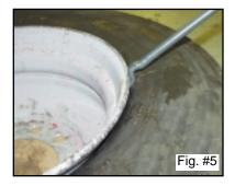
The small end of the tool easily gets under the stretched bead for that last pull.
