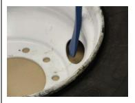
Insert spoon end into spoke hole with curved side toward the center of the wheel...
