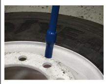
Insert knob end into lug hole on side of assembly closest to you...
