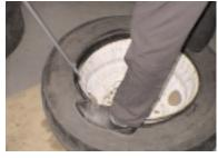
Lubricate second tire bead. Stand on the tire to push a section of the bead over the flange and into the well. While standing on the tire, insert the curved end of the tire iron between the tire bead and rim flange. Push the tire bead over the rim flange opposite where the tire is already in the well. Repeat this step taking small sections of the bead until the last section is pried over the rim flange until tire is mounted.
