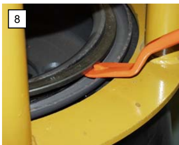
8 Push down to pry up, working around the ring until it is demounted.
