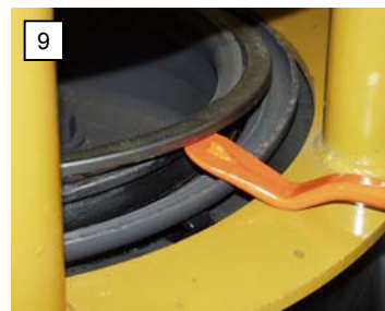
8 Push down to pry up, working around the ring until it is demounted.
