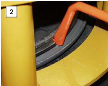
2 Insert the "toe" of the SEPARATOR end between the ends of the split ring.
