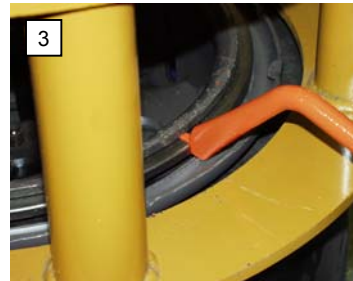
3 Push down to separate the solid ring from the split ring.
