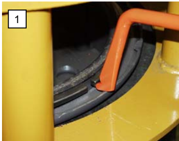
1 Locate the gap between the ends of the split ring.
