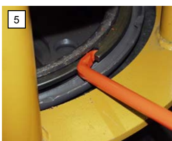
5 Pry the slotted end of the split ring out and up until it is resting against the wheel flange.
