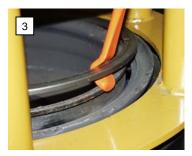
Pull the tool toward you to hook the <u>MOUNT</u> end under the ring from the inside.
