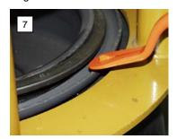
Start demounting the raised end of the split ring by placing the end of the tip of the <u>DEMOUNT</u> end under the split ring.
