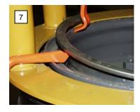
Raise the unmounted portion of the split ring using the SEPARATOR end.
