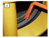
Insert the "toe" of the <u>SEPARATOR</u> end between the ends of the split ring.
