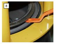
Push down to pry up, working around the ring until it is demounted.
