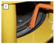
Locate the gap between the ends of the split ring.
