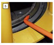
Pry the slotted end of the split ring out and up until it is resting against the wheel flange.
