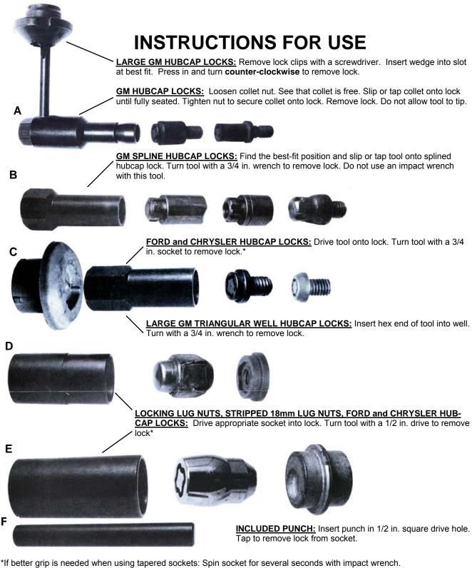
In better grip is needed when using tapered sockets: Spin socket for several seconds with impact wrench. Immediately drive socket on with hammer. Wait several seconds. Remove lock with a breaker bar. Use steady pressure. Support head of bar to keep socket from tipping. Badly worn, odd sized, or extremely stubborn locks can often be removed by lining inside of socket with a layer of medium grip emery paper, grit side in.
