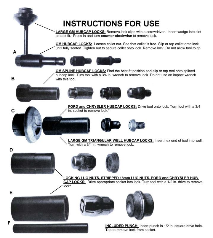
\*If better grip is needed when using tapered sockets: Spin socket for several seconds with impact wrench. Immediately drive socket on with hammer. Wait several seconds. Remove lock with a breaker bar. Use steady pressure. Support head of bar to keep socket from tipping. Badly worn, odd sized, or extremely stubborn locks can often be removed by lining inside of socket with a layer of medium grip emery paper, grit side in.
