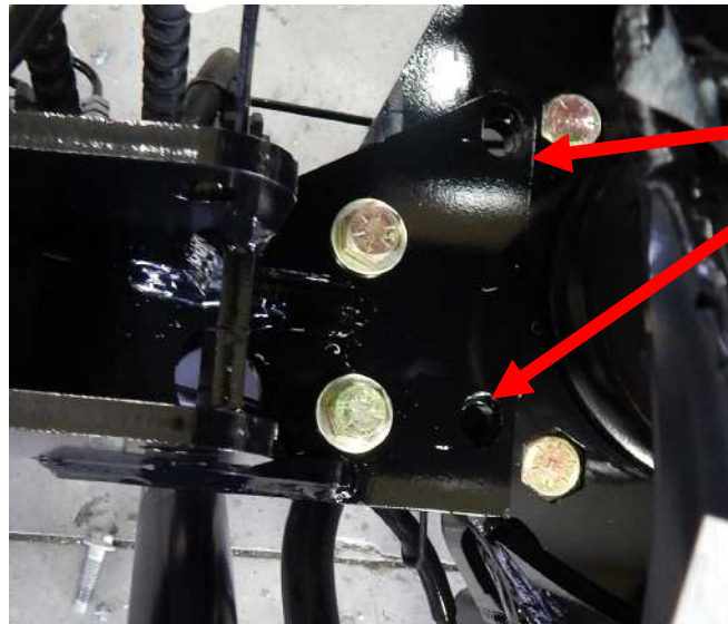
U bolts go in these holes
