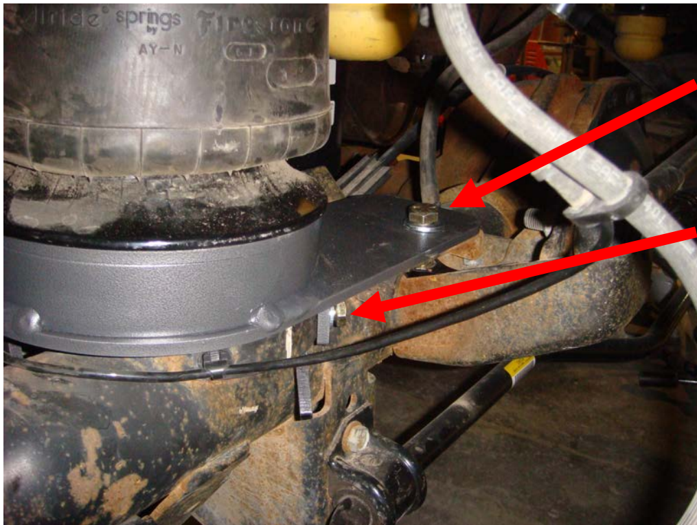
1/2 x 1 1/2" bolt uses tab nut on bottom
