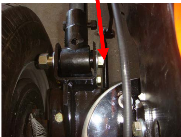
Insert bolts so the head is away from frame
