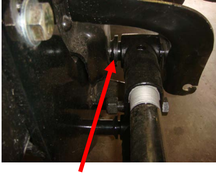
1/2" spacer goes on upper trailing arm
