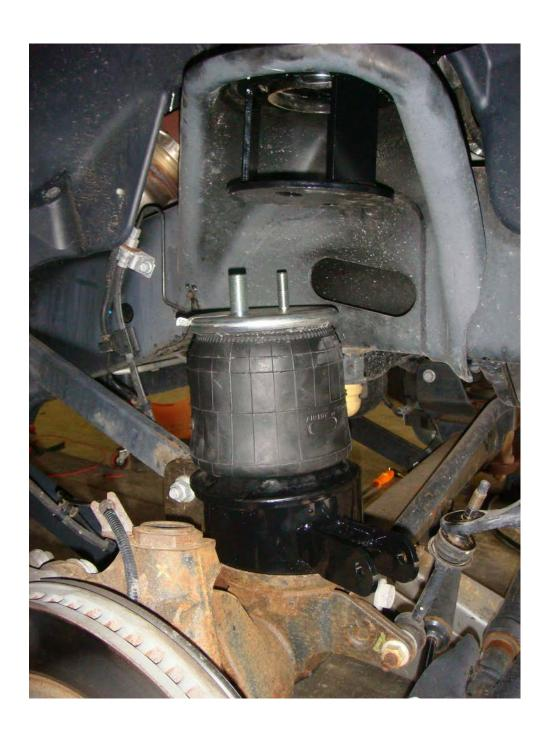
7. Once you have the air bag tightened to the lower bag mount, drop the air bag and lower bag mount into place on top of the axle. Locate the original 14mm lower shock mount and nut. Wiggle the mounting bracket in place so the holes line up and fasten in place, torqueing the 14mm bolt to 95 ft/lbs.
