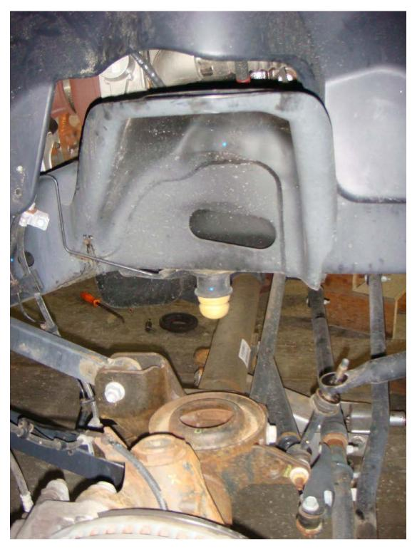
5. Locate the upper air bag mount and shock mount. The upper bag mount fits in the spring bucket. The shock mount fastens to the 3/8" studs sticking up through the spring bucket. Make sure shock mount is pointing towards the front of the truck. Install the lock washers and nuts and torque to 35 ft/lbs. NOTE: the upper bag mount should be orientated so the large hole will be away from the frame (closest to the tire).
