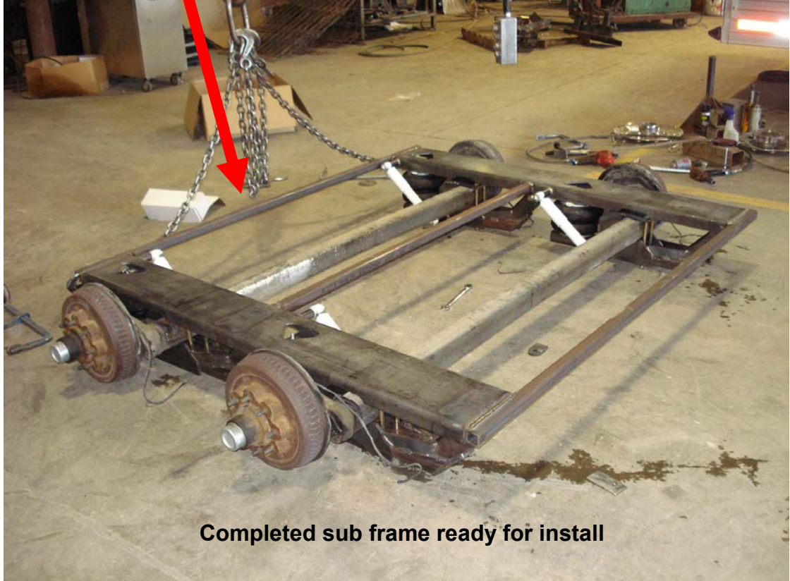
Tubing welded on the end of sub frame
