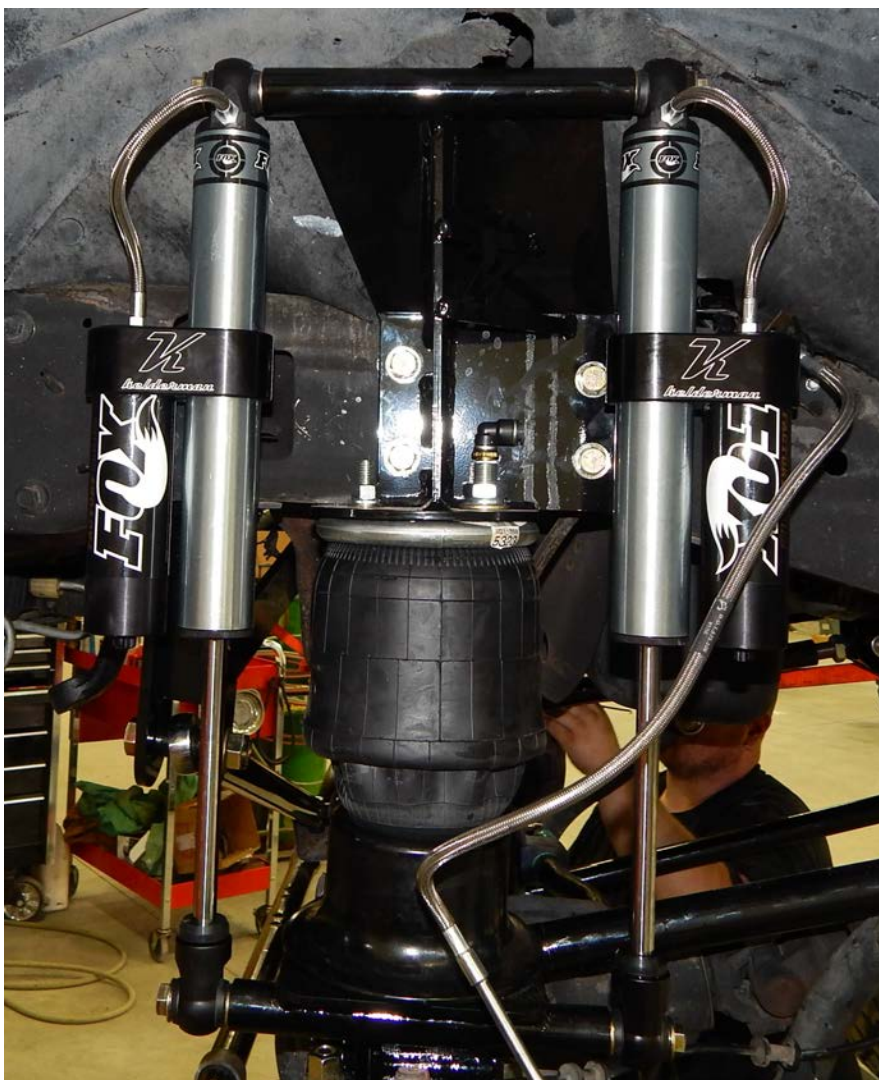
Optional Fox 2.0 Remote reservoirs shown with optional Kelderman clamps
