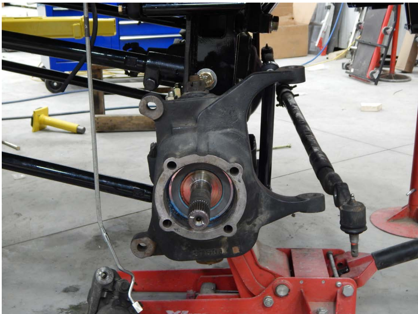
Cross over steering knuckle installed
