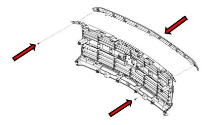
**6**: Remove four of the metal clips from the bottom of the grille frame; these will be reused during install.
