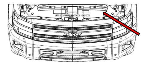
**3**: Remove the four screws that run across the top of the grille, these will be re-used during install.
