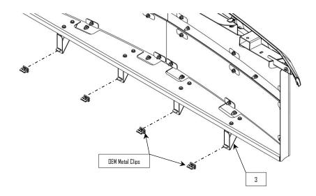
Push the four metal clips removed in *step 6* onto each of the lower tab brackets (3).
