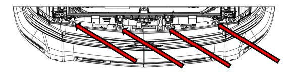
**4**: The rest of the grille is held in with clips. Carefully pull outward at each of the ten clip locations until it releases. The grille can now be removed.
