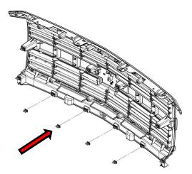
7: Remove any metal clips that may have remained clipped into the truck.
