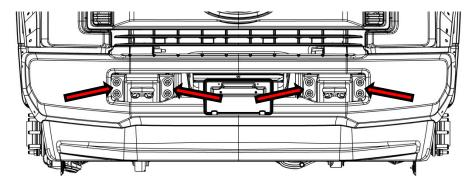
**4:** Remove the eight (8) bolts that fasten the upper bumper brackets and tow hooks to the frame. Remove the four (4) bolt tabs that fasten the lower bumper brackets to the frame. The four (4) bolt tabs will be reused during installation.
