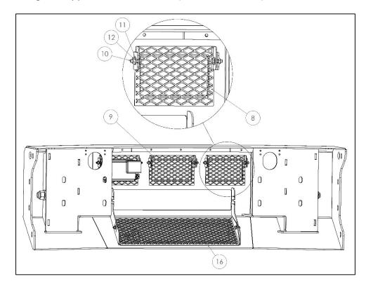
NOTE: If your truck has an adaptive cruise control sensor, install the adaptive cruise screen assembly (item 13 for 2017-2019, item 39 for 2020+) in place of the driver's side screen (8).
