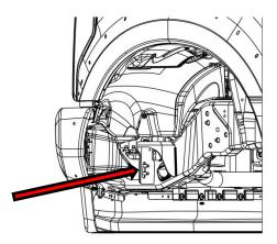
**3:** With the bumper supported remove the two (2) covers on each of the tow hooks and remove the eight (8) bolts. The bumper can now be removed.
