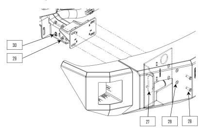
**2:** Use the studs of the bumper mount bolting tabs (27) to position the bumper on the frame brackets. Use provided  $\frac{1}{2}$ " washers and nuts (items 29 & 30) to fasten the bumper to the mount.
