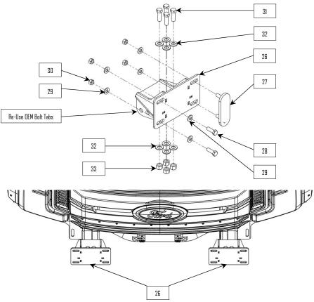
1: Install the bumper frame brackets (*item 26*). Use the provided 9/16" bolts, nuts and washers (*items 31, 32 & 33*) to bolt thru the top of the frame. Re-use the bolt tabs from step 4 in the "Bumper Removal" section to bolt thru the sides of the frame.
