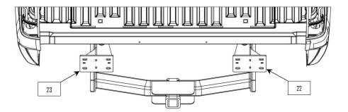
**8:** Use the studs of the bumper mount bolting tabs (5) to position the bumper on the frame brackets (22 & 23). Use washer (25) and nut (26) to fasten the bumper to the mount.
