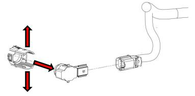
**5**: Depress the tabs on the sensor bezel and push it thru the front of bumper.
