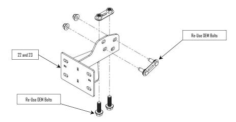
7: Install the bumper frame brackets (22 & 23). Re-use the hardware removed in steps four and five.
