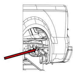
**3:** Remove the four rear bolts that fasten the receiver hitch to the frame. Save these as they will be re-used later when installing the new brackets. **NOTE:** Complete removal of the hitch is not required.
