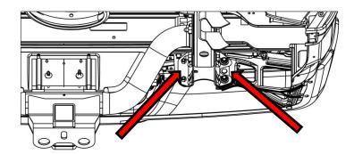
**4**: Remove the weld nuts from the four inner holes; drill these holes out to accept ½" bolts.
