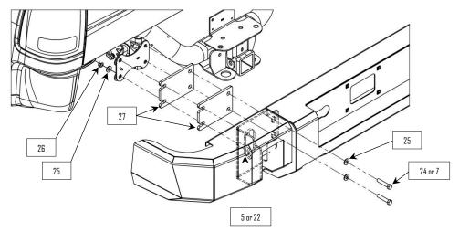
**9**: Insert the remaining ½" hardware thru the bumper and bracket. **NOTE**: Short box dually installs use the longer ½" bolts (23).
