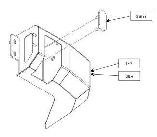
Install the tow hooks (9) into the pockets in each end cap using the provided 7/8" hardware. Tow hooks (9) and rubber washers (8) go inside the pocket. Tighten the 7/8" nut (10) to the point where the tow hook will still spin but not freely.
