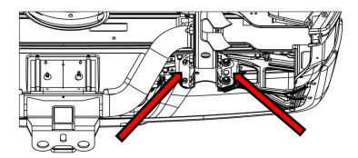
**4**: Remove the weld nuts from the four inner holes; drill these holes out to accept  $\frac{1}{2}$ " bolts.
