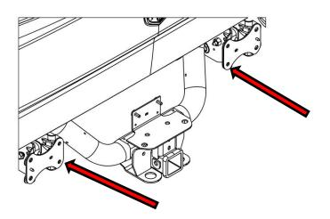
**5**: If equipped remove the parking sensors from the stock bumper **NOTE**: Keep track of location. Spread the ears on the sensor bezel and push the sensor thru the back of the bumper.
