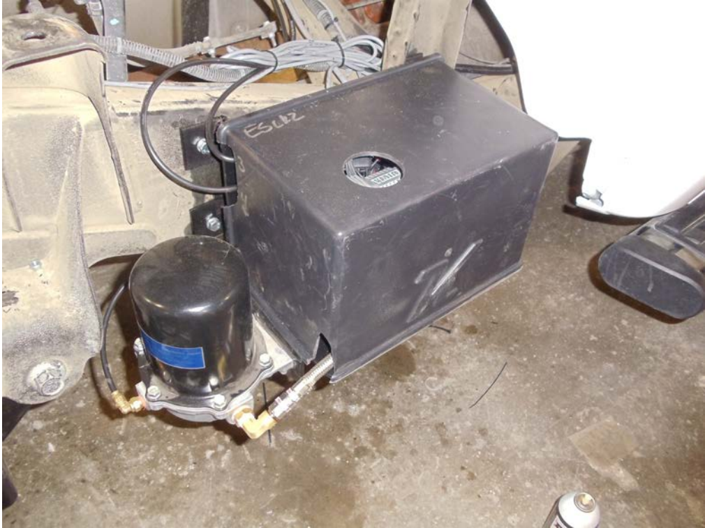
Upper forward mount fastens to the box mount closest to the cab on long box
