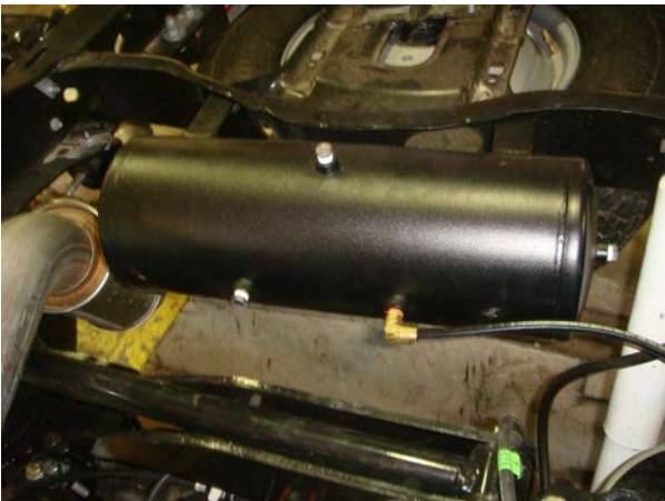
Air tank only uses one air line on the electronic system
