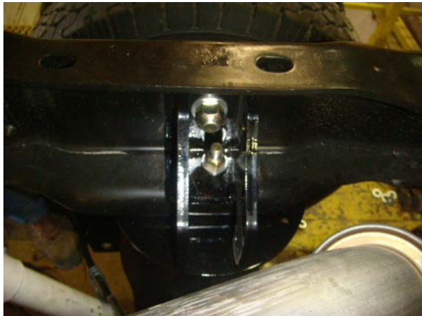
Passenger side upper air bag mount drill the front hole 1/2"
