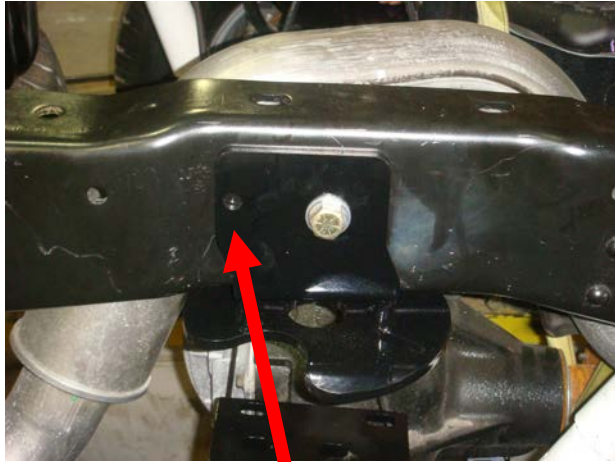
Passenger side upper air bag mount drill the front hole 1/2"
