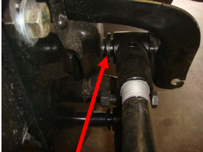
9/16 upper spacer goes on upper trailing arm
