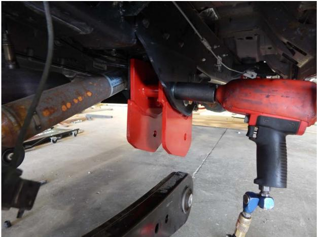
3. Remove the rear bolts that hold the factory trailing arms in place. Locate the trailing arm drops (part# 16846). They fasten into the factory trailing arm mount with four 3/4x 5 1/2" bolts. Use the picture below for placement of the bolts. Torque these bolts to 175 ft/lbs. Next, insert the factory trailing arm into the drop and fasten with the 3/4x 5 1/2" bolts. Torque this bolt to 175 ft/lbs also. Do both sides at the same time.
