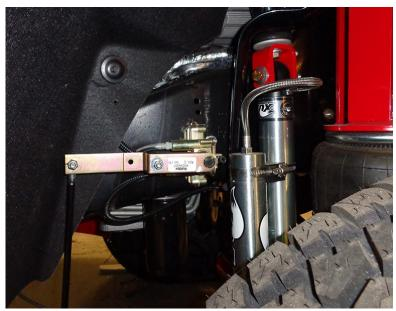
The mechanical valve at ride position. Note the arm is straight. Before installing rotate the arm 3 turns each way to get the internal parts ready for operation. The top port is exhaust, the bottom port is input from tank and middle port is out to air bags.
