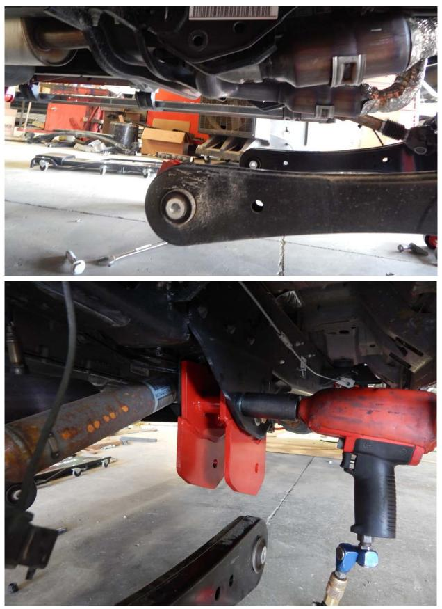
3. Remove the rear bolts that hold the factory trailing arms in place. Locate the trailing arm drops (part# 16846). They fasten into the factory trailing arm mount with four 3/4x 5 1/2" bolts. Use the picture below for placement of the bolts. Torque these bolts to 175 ft/lbs. Next, insert the factory trailing arm into the drop and fasten with the 3/4x 5 1/2" bolts. Torque this bolt to 175 ft/lbs also. Do both sides at the same time.
