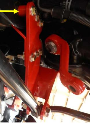
5. Locate the pan hard bar (track bar) drop bracket (part# 16847) with backing plate, (part# 15381). Install the pan hard bar drop and backing plate with the supplied bolts and spacers. Use the pictures below for bolt placement. NOTE: The button head bolt goes in the hole closest to the air bag. Make sure the smooth head is on the bottom of the frame with the nut and threads on the inside of the frame. Torque the M20 bolt to 150 ft/lbs and the 1/2" bolts to 85 ft/lbs
