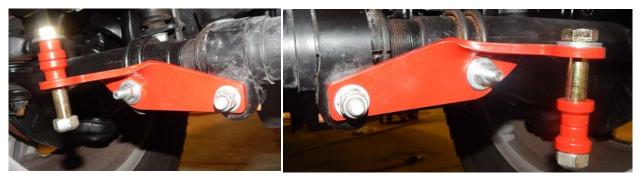
9. Locate the upper shock mounts (part# 17139). They fasten into the original upper shock hole in the spring bucket. Remove the upper rubber mounting brackets from the factory shocks and use them and the M12x70 to fasten into place. Insert the bolt so the threads are up. Torque this bolt to 65 ft/lbs. Now install the shocks with the 1/2x3" bolts. Torque these bolts to 85 ft/lbs. Depending on what brand of shock is used, you may need spacers or washers to center the shock.
