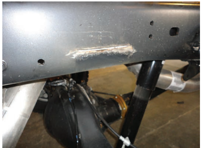
Below, Right—Bump stop shown removed.
