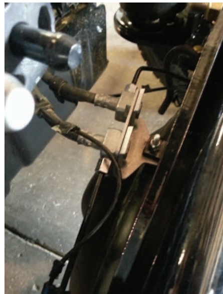
Below, Right—Brake Line Tab shown mounted on rear of differential.
