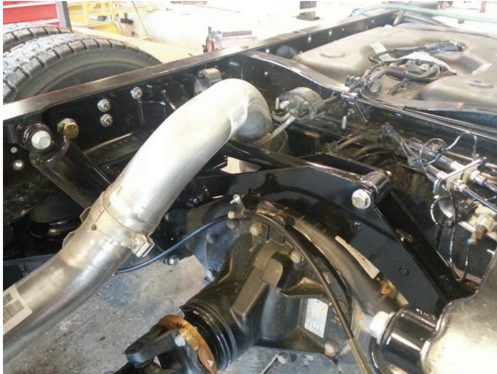
Above Photo—Completed installation of crossmember, pan hard bar and exhaust hanger.
