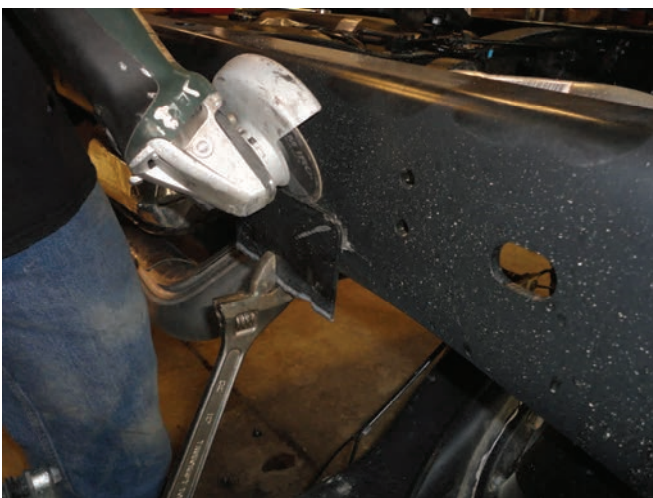
Grinder shown removing bump stop.
