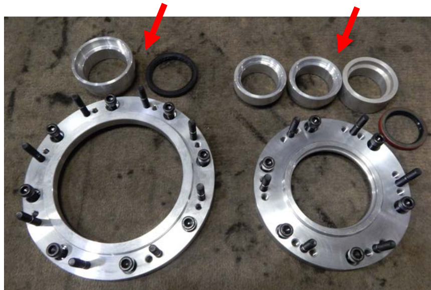
6 bolt indexing ring and 3 different seal adaptors for manual and automatic transmissions
