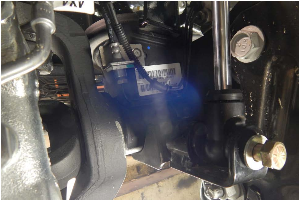
Make sure the knuckles have the gussets towards each other
