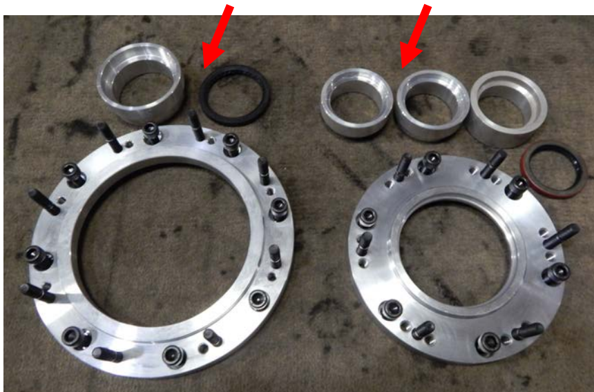
6 bolt indexing ring and 3 different seal adaptors for manual and automatic transmissions
