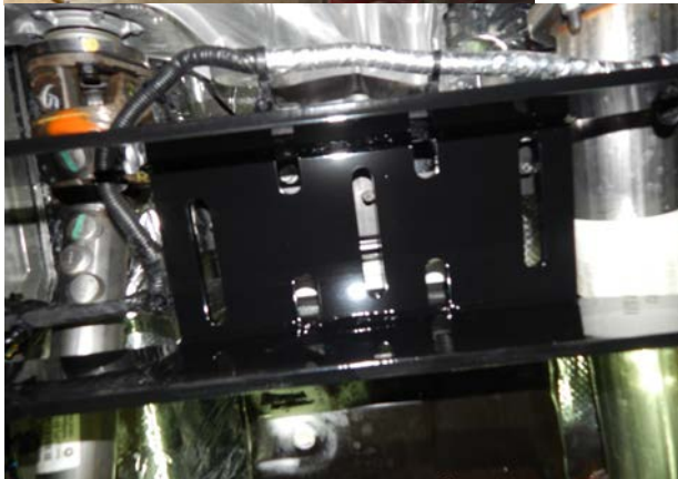
Knuckles should be installed with the gussets facing each other, as shown in the photo.
