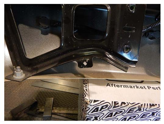
9.) With the leaf spring perches removed, locate the upper framework of the 2-Stage Rear Air Suspension. Remove the (3) factory 14mm bolts from each side of the factory hitch framework. The upper framework will fasten into the frame/hitch assembly with these 14mm x120 bolts. Torque these bolts to 115 ft./lbs.
