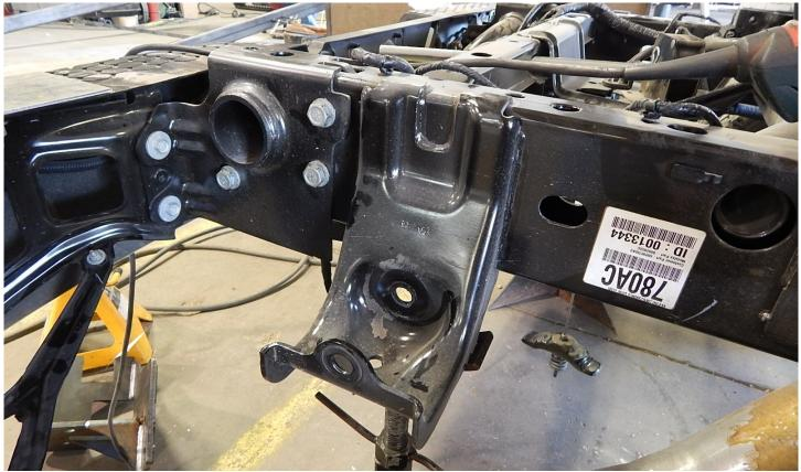
6.) Using a torch, saw or a plasma cutter, remove the shackles from the frame as shown in the photo below. **DO NOT CUT INTO THE FRAME.** The leaf springs do not have to be removed for the installation of this kit.
