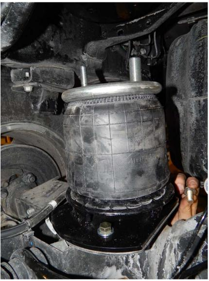
4. Now that the air suspension is installed, reconnect the factory end links to the sway bar and reconnect the lower shock bolt.
