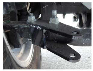
3. Locate the drivers side bracket (Part # 18839 and 18397) If fastens to the two factory pinch bolts on the steering arm. It also fastens to the outer tie rod end with the  $1/2 \times 3$ " bolts. Torque these bolts to 55 ft./lbs. Make sure the 1/2" bolt is pointing towards the rear of the truck.
