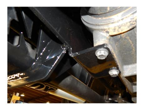
5. Locate the shocks. (Fox Part # 985-24-068). Use the  $1/2 \times 3$ " bolts on the outside to fasten the shock to the outer mounts. Locate the shock strap (Part # 18402 and two  $1/2 \times 3$ " bolts. Fasten the shocks to the steering stabilizer bracket. Make sure to put the bolts in from the top down. Once all the bolts are in place, go back and torque the bolts to 75 ft./lbs.
