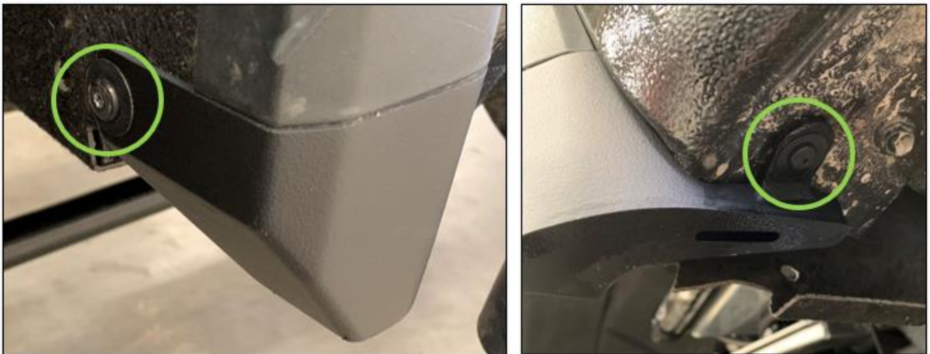
Figure 4: Kelderman fender flare cap installation points
