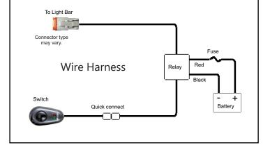
the relay using the supplied sheet metal screw. Attach the negative (black) wire to a good chassis ground and power (red) wire to a positive 12 volt power source.
