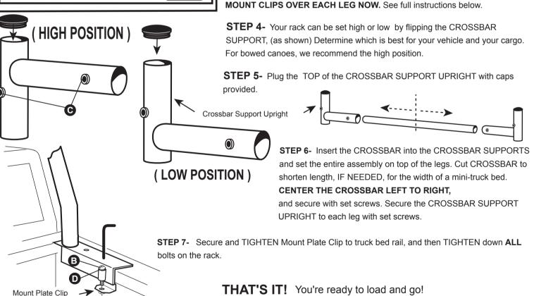
• If you are installing an ECONO TRUCK RACK on the back of your truck bed, repeat the above. Before drilling the mounting plate, make sure that the plate dose not overhang or interfere with the tail gate. Before inserting the Caps, make sure that the height setting in the rear matches the height setting in the front.
