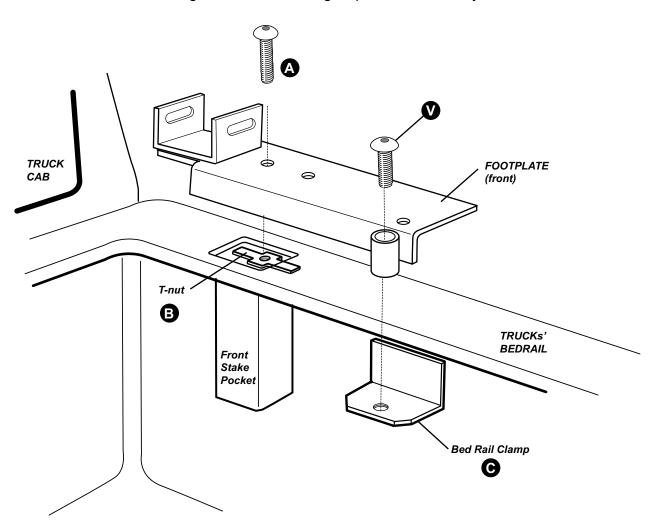
**#1=** Lift the rack up onto the truck bedrail. Loosely attach the front legs to the secured FRONT FOOTPLATES as shown in **STEP 7**. Position the REAR FOOTPLATES against the bedrail. Attach the REAR FOOTPLATES to the truck bedrail using bedrail clamps as shown in the illustration.
