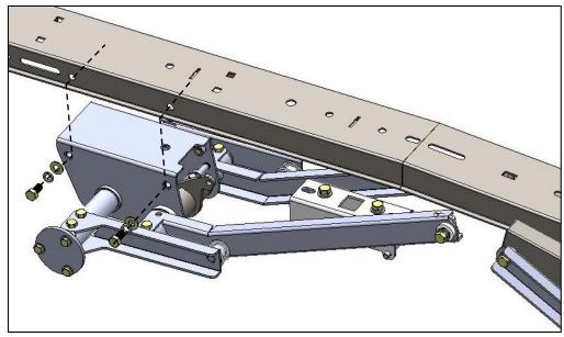
Bolt "Torque tube pivot Assy. 2(40993-8)" underneath the rearcrossbow (rear side of the vehicle) as shown below using 3/8"x3/4 Bolts with flat and lock washers. You may need to un-bolt the mounting front from the crossbow to do this.
