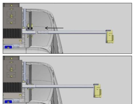
Next attach the "Ladder Hooks (40800-31)" and "Ladder Stops (40900-30-004)". Attach "Ladder Hooks" to ladder pans on 5/16" studs in desired location. Attach "Ladder Stops" to coincide with "Ladder Hooks" by removing 3/8"x3/4" bolt and placing stop so the tab on the stop goes into the corresponding slot. If using a "step ladder" mount "Ladder Hooks" in the upper location in the rear. If you are using an "extension ladder" use the same location as the front bow.
