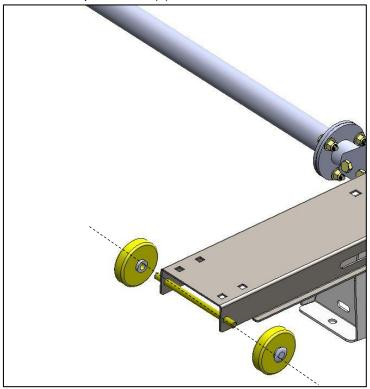
Next install the "Ladder Pan Assy." Align cutouts in "Ladder Pan Assy. (40993-10)" with the "Rollers" and guide the arms onto the "Torque Tube Pivot Assy." As you lower the Pan assembly onto the rollers, remove the bolt assembly pre-installed on Ladder Pan, and use the same bolt assembly to secure the Arm with Ladder Pan. Caution: Make sure the nylon spacer is sandwiched between the Arm and Ladder Pan, and lock washer or nyloc nut is used on this assembly.
