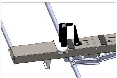
First using 5/16"x1.5" Hex bolt (q) with two flat washers(b) and nyloc nut (d) to connect the ladder pan stiffener (40993-31 and 40993-832) and USE E6000(m)AROUND HOLES. Attach ladder pan stiffener, in the closed position, using 5/16"x5/8" bolts (e) with lock washers (c) and flat washers (b). Confirm that distance between passenger side feet and driver side feet are still EXACTLY the same. Now you can tighten the feet for the front and rear bow assemblies.
