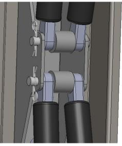
Attach torque tube(40993-25 and 40993-24) using ½" bolts (J) with flat washers(k) and nyloc nuts(l). Check distance between feet on both driver and passenger side, they must be EXACTLY the same to insure the bow assemblies are parallel.
